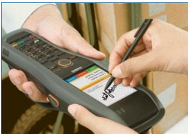
The 3,5 inch transfective colour LCD is produced by CASIO. A user friendly data input and signature capturing method can be done with the touch pen and scratch-resistant touch screen of the device. No matter if glaring sunlight or night delivery – the graphic display with 240x320 pixels is readable under all light conditions.
